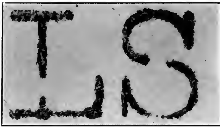
FIG. 188—Defective letters on a new machine.
